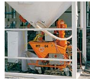
Direct connection to silo
